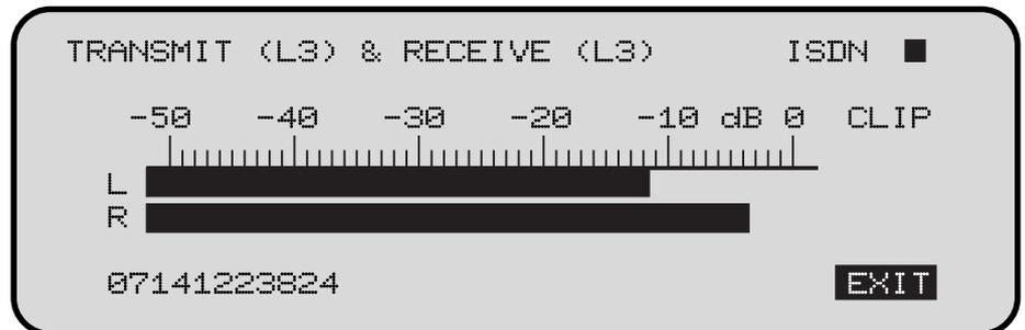
The peak level is indicated, related to the maximum level at the input of the A/D converter. Overmodulations (CLIP) should be avoided on all accounts.
